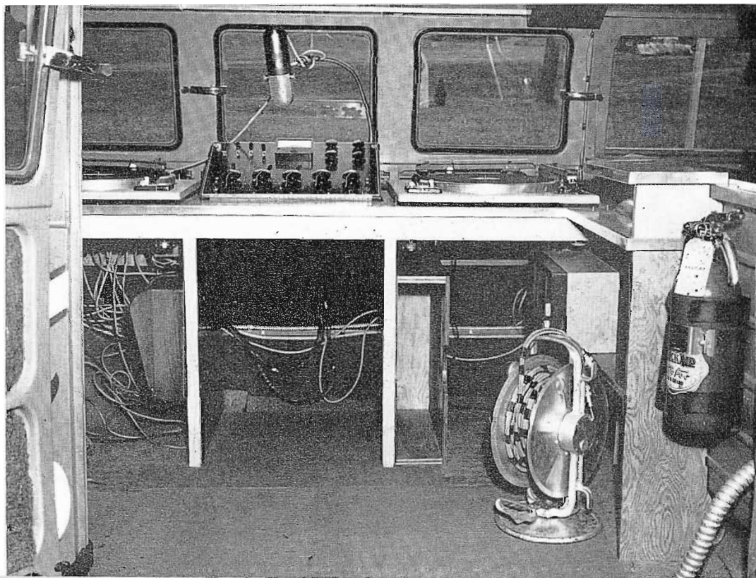
FIG. 5. Custom built table and shelves to house the D-J studio line one side of the mobile unit.
