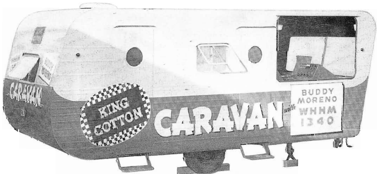
FIG. 21. This is a typical mobile studio of the type employed for remote broadcasting. (Shown here is the WHHM mobile unit with BC-5A audio-consolette inside.)
