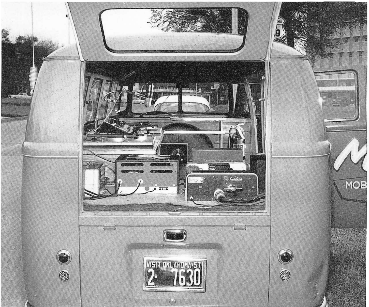
FIG. 2. Rear view of KRMG Mobile Studio. Note two-way radio "Carfone" unit at right.
